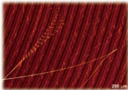
The electron micrograph shows a metallic glass nanowire that involves ultrahigh strength and high elasticity. The sine wave pattern demonstrates the vibration of the nanowire.
