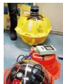
There are seismometers installed at the end of a tunnel that was constructed 44 years ago, located 45 meters underground and accessed by elevator at RCPEV.
