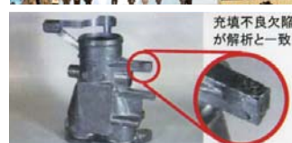
A practical casting throttle chamber and results of flow analysis
