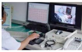
Images are highly compressed, while maintaining high definition, so that a doctor at a distance from a patient can check the patient's face complexion, presence of skin diseases, edema, actions, way of walking, etc. In addition, diagnostic data is encrypted to prevent any leak of a patient's personal information, and transmitted to doctors at a hospital/clinic via a PHS or a mobile phone.
