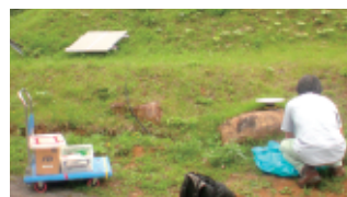
A disk-shaped device in front of a person is a GPS receiving antenna, and a rectangular device on the bank slope in the back is solar panels to supply power. These solar cells make it possible to acquire data during the power outage caused by the earthquake.
