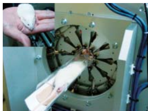
Small animal semiconductor PET that has a high spatial resolution of less than 1 mm FWHM for the first time in the world. This makes it possible to do biomedical experiments with mice.
