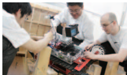
Kenaf (a tracked vehicle for exploration). This is remotely operated from a safe place by means of wireless LAN, and is capable of measuring 3D shapes.
