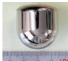
New Zr-based bulk metallic glass (a maximum diameter of 30 mm)
