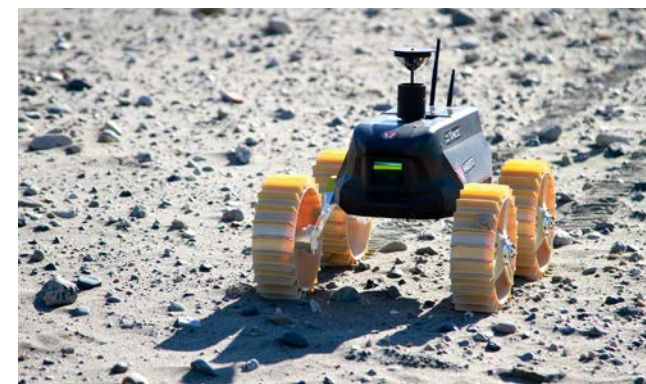
MoonRaker(4-wheel rover) in field tests over a sand dune in Japan ©Tohoku University/team HAKUTO
