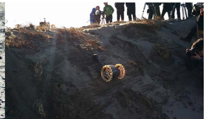
Tetris(2-wheel rover) in down-cliff tests hanging by tether from Moonraker ©Tohoku University/team HAKUTO
