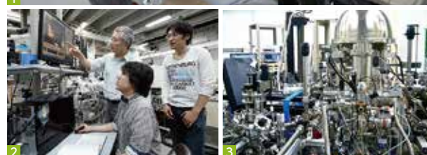
[Photo 1 2 3] In Professor Takahashi's laboratory, the ultrahigh-resolution spin-resolved photoemission spectrometer was constructed to study the spin state of materials. The machine achieves the world-best resolution of 8meV.
